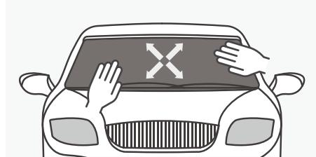
**8** Remove the J&J solution with squeegee to fix the film.
