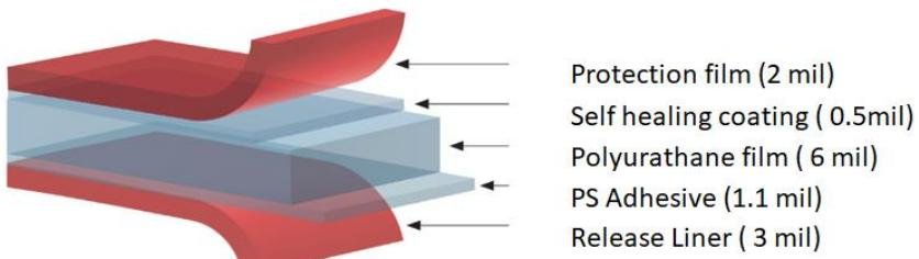
Nominal Thickness (Polyurethane film+ PSA+ SH Coating):  $180 \pm 10\%$
